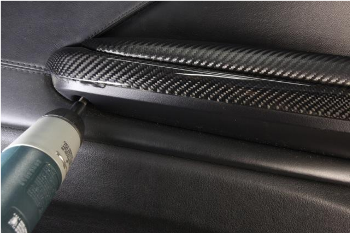
Remove the screw under the arm rest near the rear using a Torx 20 bit.
