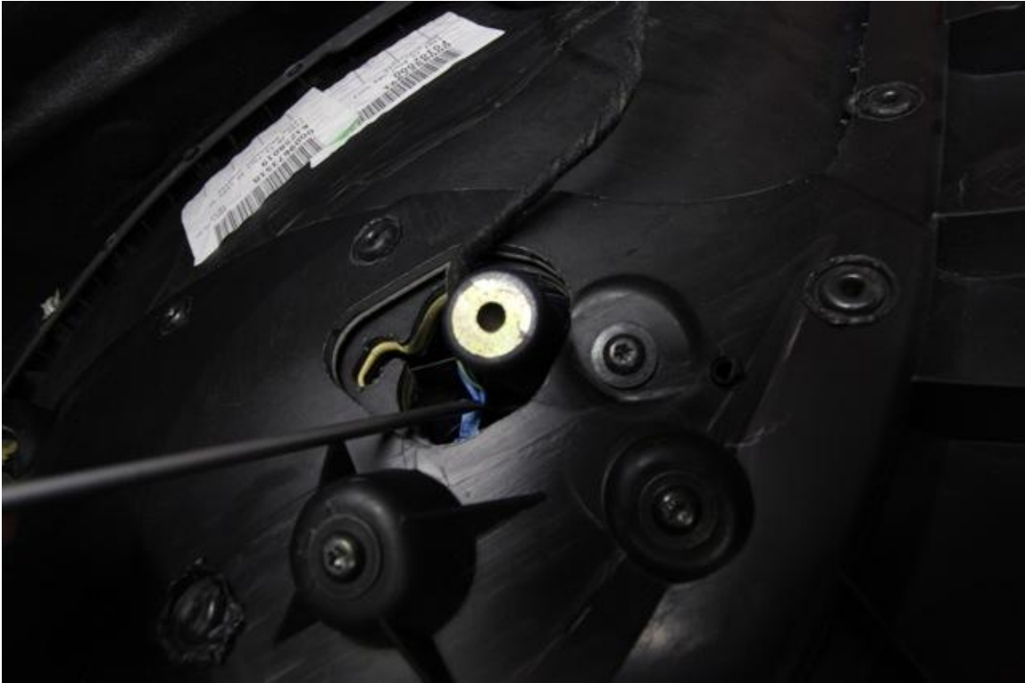
Release the mirror controls from the panel by using a small flat head screw driver and unclipping the blue connector.
