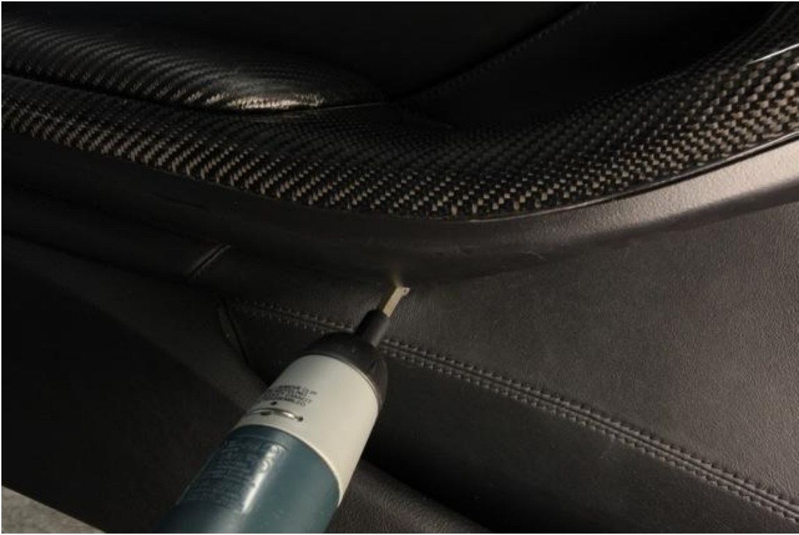
Remove the screw under the arm rest near the middle using a Torx 20 bit.
